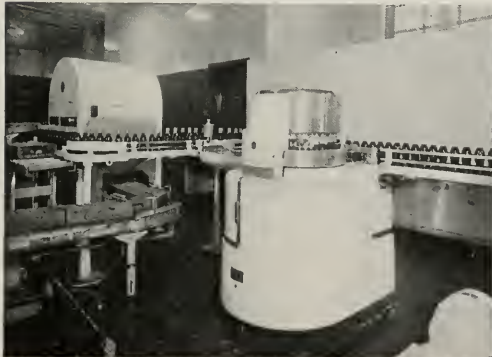
FOREIGN OBJECTS IN BOTTLED DRINKS ARE INSTANTLY DETECTED BY THIS ELECTRONIC BEVERAGE INSPECTOR WHICH AUTOMATICALLY REJECTS IMPERFECT PRODUCTS.
