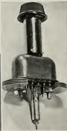
THIS 4,000 MEGACYCLE MAGNETRON CAN BE TUNED FROM THE OUTSIDE WITHOUT AFFECTING THE STABILITY OF THE TUBE.
